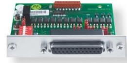
The R&S H0118 binning interface enables use with external hardware that sorts components by physical type after measurement. Data lines for eight sorting containers and control lines (ALARM, INDEX, EOM, TRIG).
