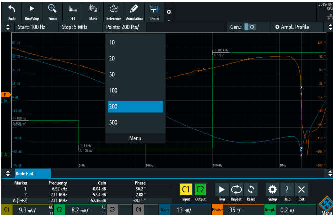
The measurement resolution can be varied by changing the points per decade
